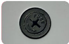
The fuse holder is located on the bottom of the device.
